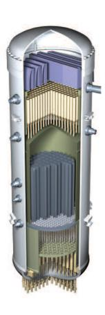
The ESBWR (Economic Simplified Boiling Water Reactor) builds on a long line of proven GEH BWR reactors. ESBWR employs passive safety design features. It is a simplified reactor design, allowing faster construction and lower costs.
