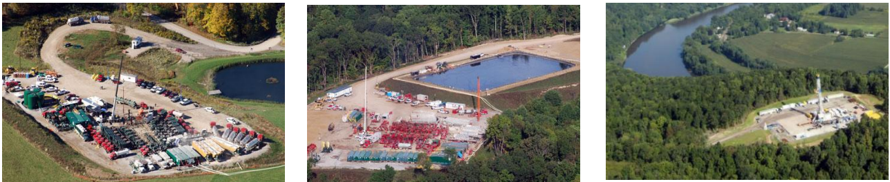
Fig. 9. Typical Fracking Well Pads in the US. A holding pond of 0.5 – 1.0 ha is needed to store the return water before treatment.
